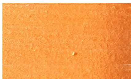
Figure 2. Cotton threads after dyeing with Bixa Orellana treated with an alkali solution.
